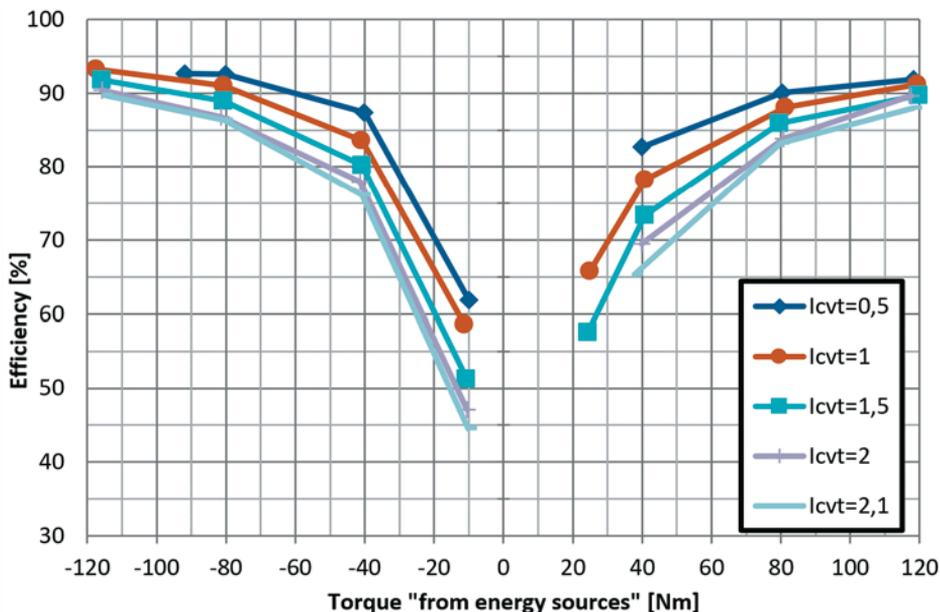
Fig. 9. Efficiency of the tested continuously variable transmission
