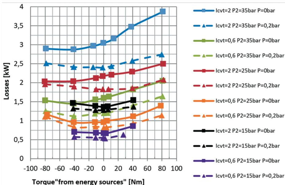
Fig. 5. The effect of lowering the oil level on losses
