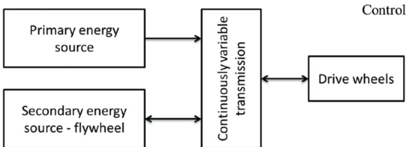
Fig. 3. The idea of a prototype hybrid drive system
