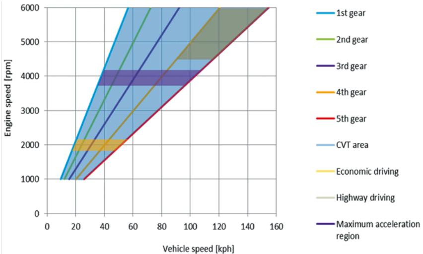
Fig. 2. The transmission range of the continuously variable transmission compared to a conventional five-speed transmission
