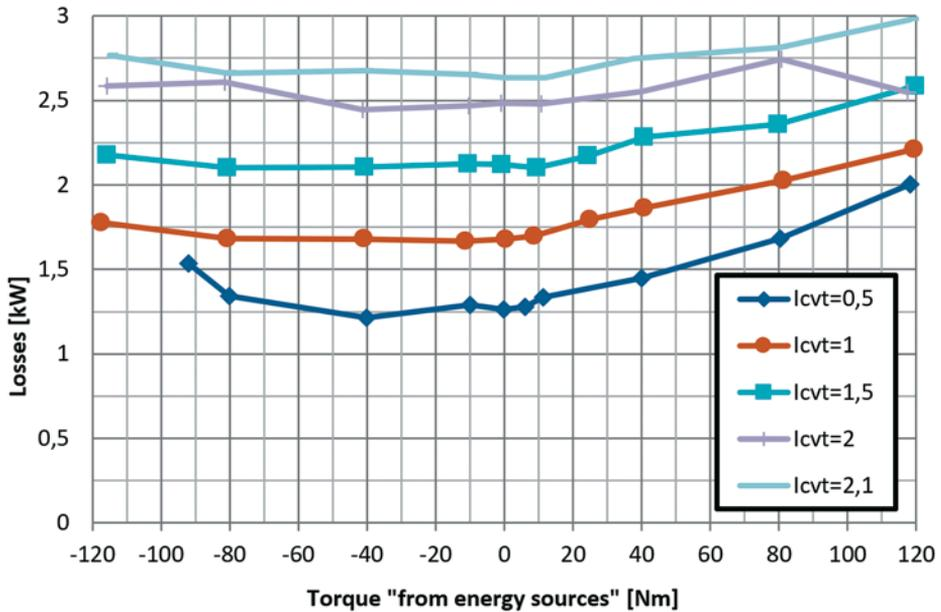
Fig. 6. Losses generated by a continuously variable transmission
