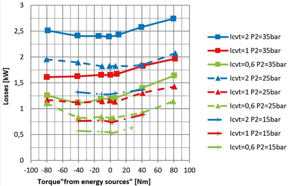
Fig. 7. The effect of P2 pressure reduction on losses
