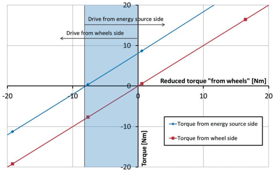
Fig. 8. Comparison of moments on both sides of the transmission
